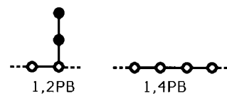
Figure 1. United atom structures for 1,2- and 1,4-polybutadiene (PB) monomers. Open circles denote united atom groups belonging to the chain backbone, while filled circles indicate the side groups.
